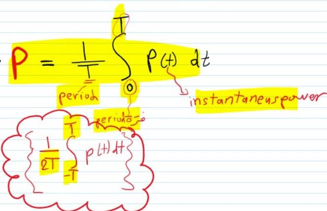
$$P = V_{\text{rms}} I_{\text{rms}} \cos(\phi_v - \phi_i)$$
