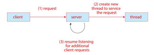
Figure 4.2 Multithreaded server architecture.
