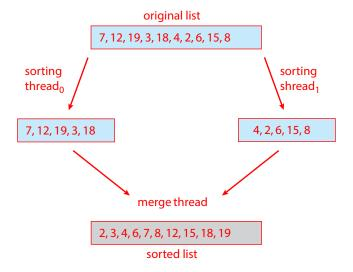
Figure 4.27 Multithreaded sorting.
