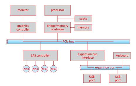
Figure 12.1 A typical PC bus structure.
