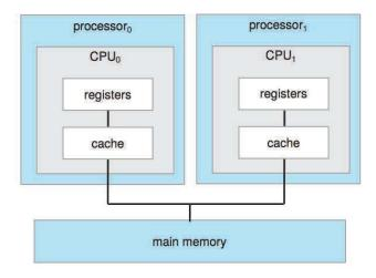
Figure 1.8 Symmetric multiprocessing architecture.
