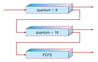
Figure 5.9 Multilevel feedback queues.
