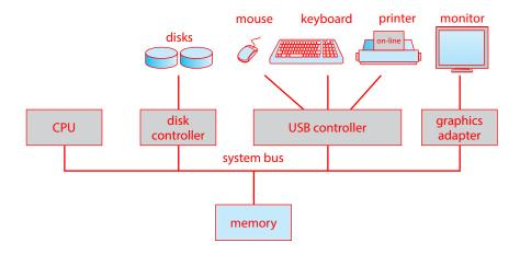
Figure 1.2 A typical PC computer system.
