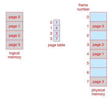
Figure 9.9 Paging model of logical and physical memory.
