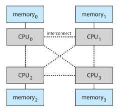
Figure 10.19 NUMA multiprocessing architecture.
