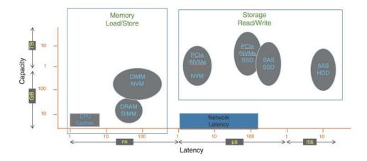
Figure 12.18 I/O performance of storage (and network latency).
