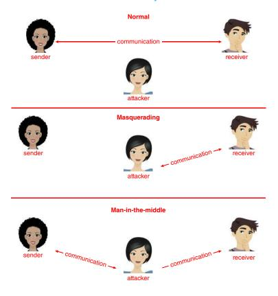
Figure 16.6 Standard security attacks.<sup>1</sup>
