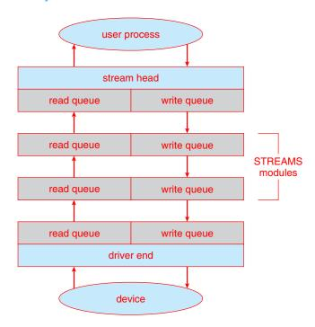
Figure 12.15 The STREAMS structure.
