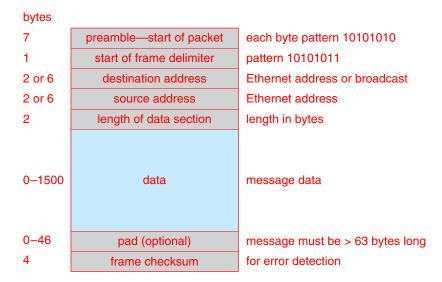
Figure 19.9 An Ethernet packet.
