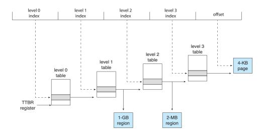
**Figure 9.27** ARM four-level hierarchical paging.
