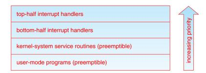
Figure 20.2 Interrupt protection levels.
