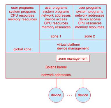
Figure 18.7 Solaris 10 with two zones.
