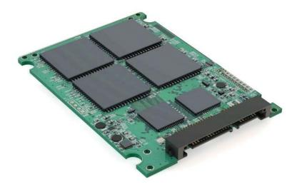
Figure 11.3 A 3.5-inch SSD circuit board.
