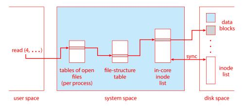
Figure C.8 File-system control blocks.
