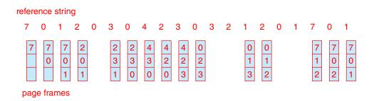
Figure 10.12 FIFO page-replacement algorithm.
