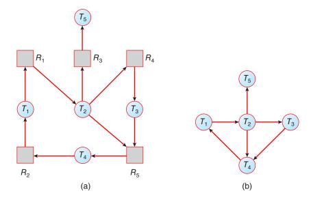
**Figure 8.11** (a) Resource-allocation graph. (b) Corresponding wait-for graph.
