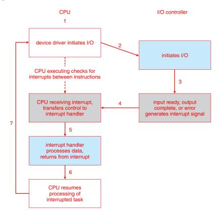
Figure 1.4 Interrupt-driven I/O cycle.
