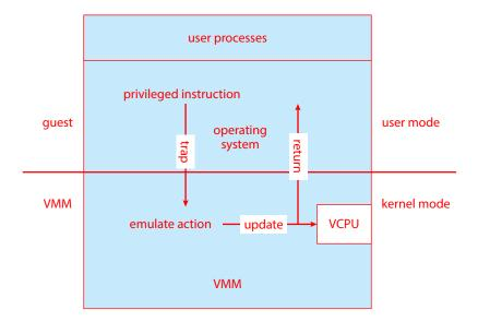
**Figure 18.2** Trap-and-emulate virtualization implementation.
