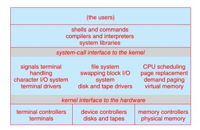
**Figure C.2** 4.4BSD layer structure.
