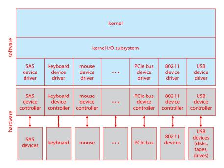
Figure 12.7 A kernel I/O structure.
