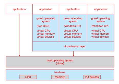
Figure 18.9 VMware Workstation architecture.
