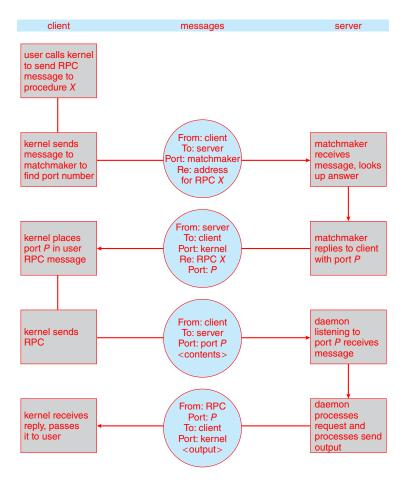
Figure 3.29 Execution of a remote procedure call (RPC).
