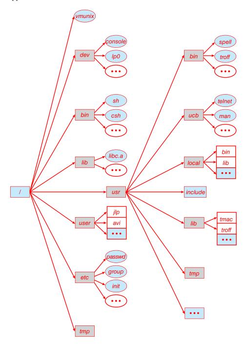
Figure C.3 Typical UNIX directory structure.
