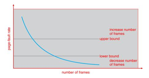
Figure 10.23 Page-fault frequency.
