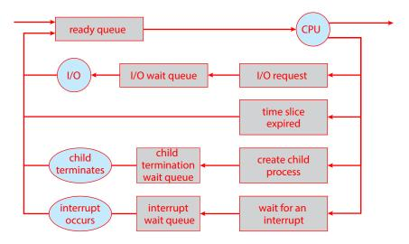
Figure 3.5 Queueing-diagram representation of process scheduling.
