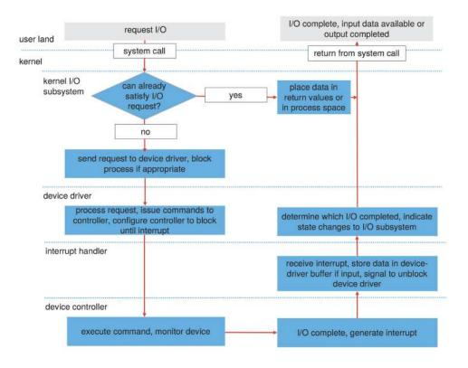
Figure 12.14 The life cycle of an I/O request.
