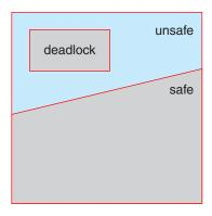
Figure 8.8 Safe, unsafe, and deadlocked state spaces.
