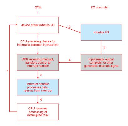
Figure 12.3 Interrupt-driven I/O cycle.
