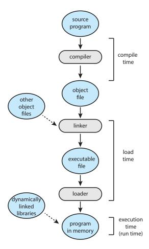
Figure 9.3 Multistep processing of a user program.
