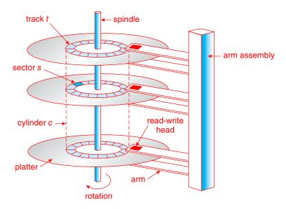
Figure 11.1 HDD moving-head disk mechanism.
