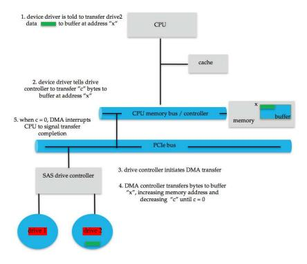
Figure 12.6 Steps in a DMA transfer.
