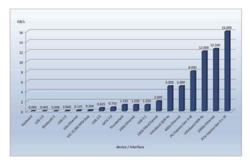
Figure 12.11 Common PC and data-center I/O device and interface speeds.
