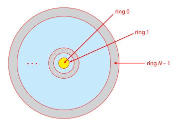
Figure 17.1 Protection-ring structure.
