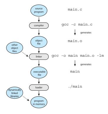
Figure 2.11 The role of the linker and loader.
