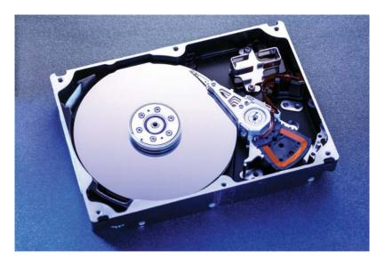
**Figure 11.2** A 3.5-inch HDD with cover removed.
