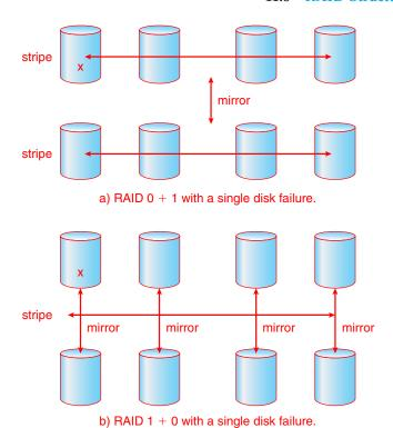
Figure 11.16 RAID 0 + 1 and 1 + 0 with a single disk failure.
