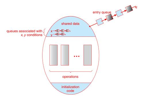
Figure 6.13 Monitor with condition variables.
