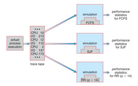
Figure 5.31 Evaluation of CPU schedulers by simulation.
