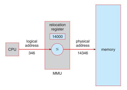
**Figure 9.5** Dynamic relocation using a relocation register.
