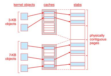
Figure 10.27 Slab allocation.
