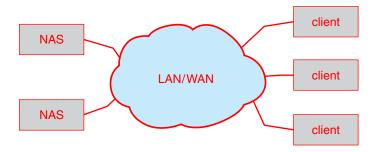
Figure 11.12 Network-attached storage.
