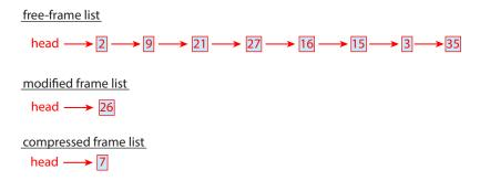
Figure 10.25 Free-frame list after compression
