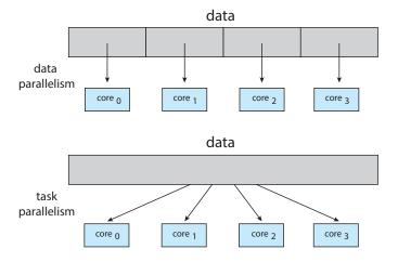
Figure 4.5 Data and task parallelism.
