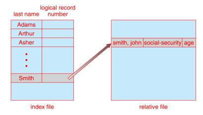
Figure 13.6 Example of index and relative files.
