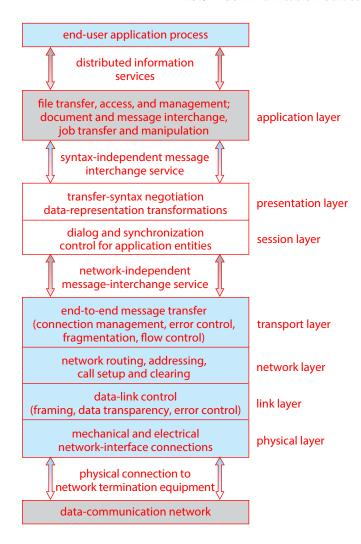
Figure 19.6 The OSI protocol stack.
