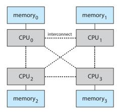
Figure 1.10 NUMA multiprocessing architecture.
