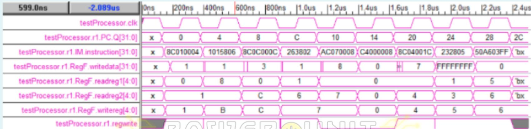
Given that the above timing diagram is for the single cycle processor in experiment 6, answer the below true or false questions.
