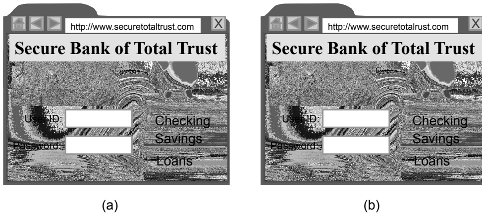
Figure 14: A phishing attack based on a misspelled URL, which could, for example, have been included in a spam email asking a customer to check their account balance: (a) The real web site . (b) A phishing web site.
