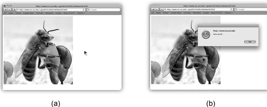
Figure 9: A mouse-over event that triggers a Javascript function, using the Apple Safari browser: (a) Before the mouse-over event. (b) After the mouse-over event.
