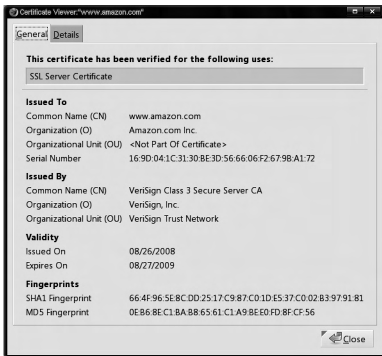
Figure 5: A web server certificate as displayed by Firefox. The fields of the certificate include the name of the organization owning the web site, the domain name of the website, the name of the CA that issued the certificate, the expiration date, and cryptographic parameters.
