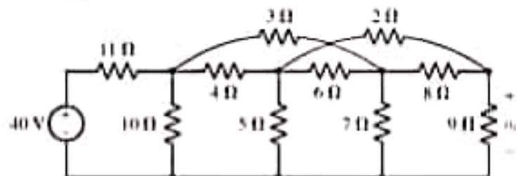
Q2: Find the value of the resistance to be connected on the open circuit terminal to absorb the maximum power and determine the value of the absorbed power.
