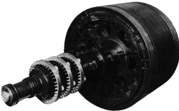
FIGURE 6–4 Typical wound rotors for induction motors. Notice the slip rings and the bars connecting the rotor windings to the slip rings. (Courtesy of General Electric Company.)
