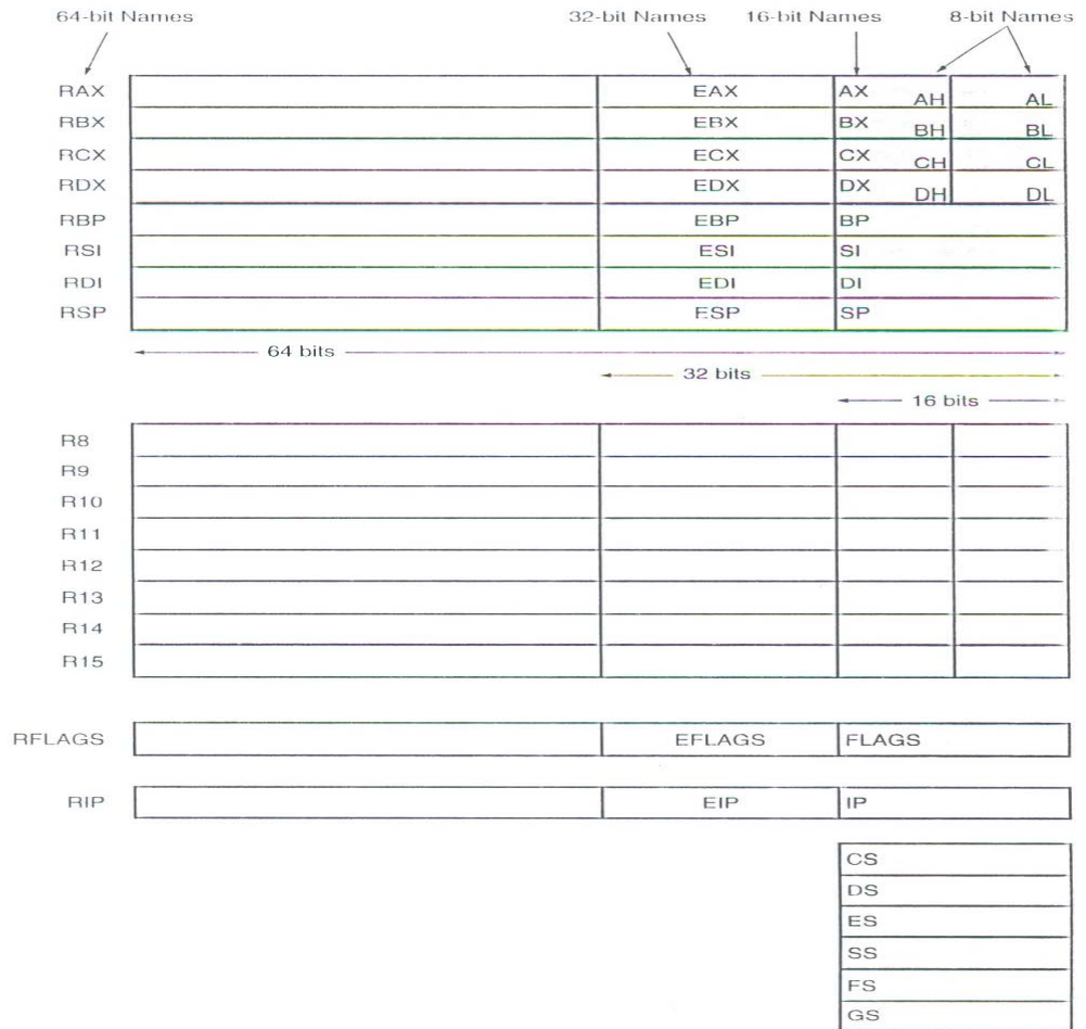
FIGURE 2-1 The programming model of the 8086 through the Core2 microprocessor including the 64-bit extensions.
