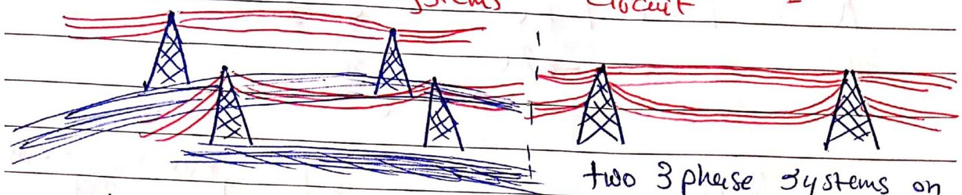
two 3 phase systems on two different towers / transmission lines.
