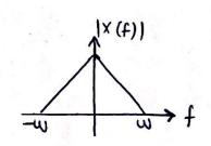
Sampling - Repeat the signal (spectrum) around the sample freq (fs)
