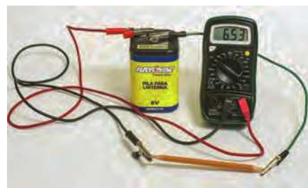
Figure 11.46 ▲ Demonstration of the electrical conductivity of graphite The nonzero reading on the meter shows that the pencil lead (graphite) conducts electricity.
