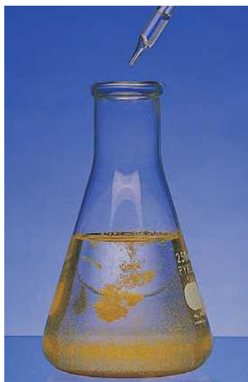
Figure 17.2 ▲ Demonstration of the common-ion effect When the experimenter adds lead(II) nitrate solution (colorless) from the dropper to the saturated solution of lead(II) chromate (pale yellow), a yellow precipitate of lead chromate forms.
