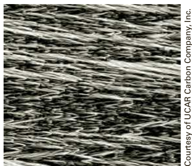
Figure 11.45 ▲ Electron micrograph of graphite Note the layer structure.
