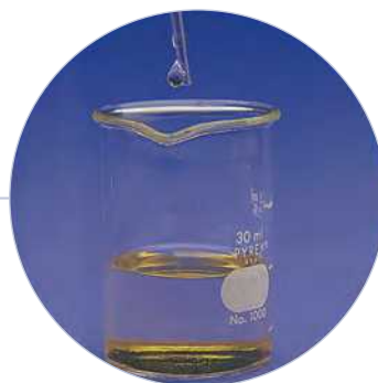
Figure 3.5 ◀ Preparing resorcinol-formaldehyde plastic
