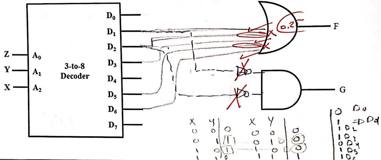
**Problem 5.** Given the following implementation of the function  $F(X, Y, Z)$ , write the minterms of  $F$  in the equation below. (2 points)
