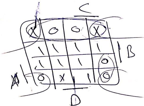
$$\bar{f} = \bar{A}\bar{B} + \bar{B}\bar{D} + AC\bar{D}$$
