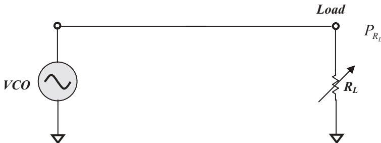
Figure 6.32 VCO load pulling test.
