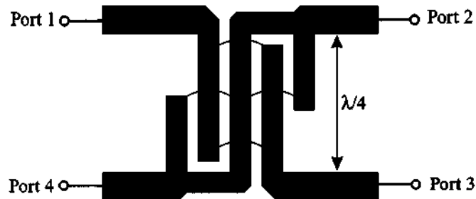
Figure G-7 A 3 dB Lange coupler.
