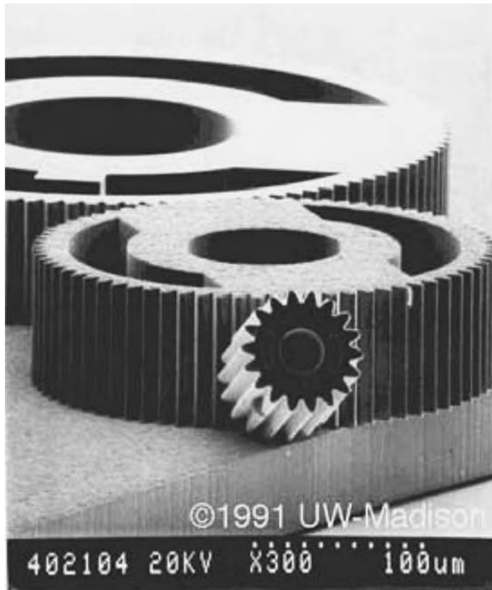
FIGURE 5.7 These three gears are examples of structures that were built with the LIGA process. See http://mems.engr.wisc.edu/images/gears/ .
