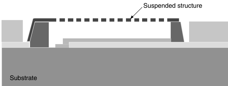
FIGURE 5.6 Example of surface micromachining. The structure is built up on the substrate surface. (Courtesy of Raytheon.)
