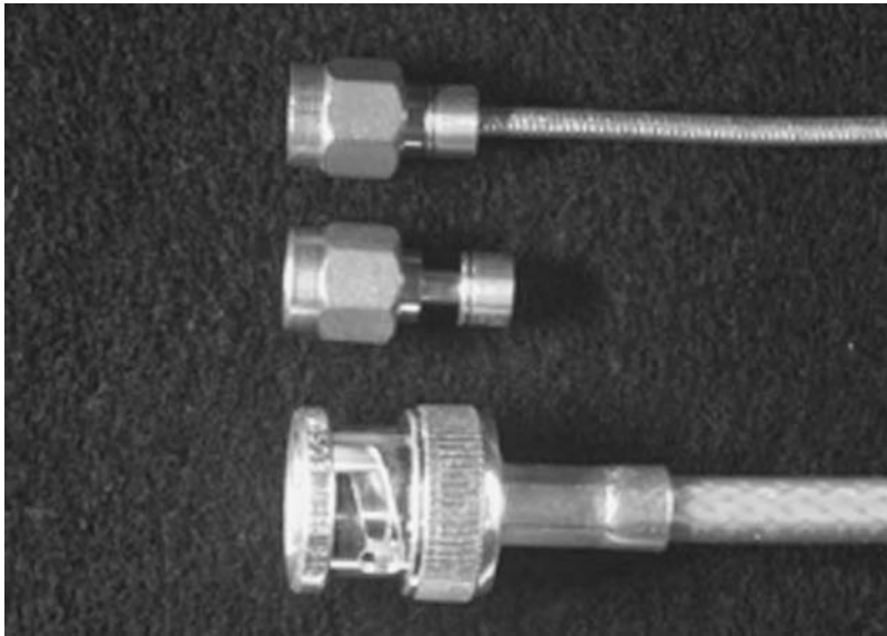
FIGURE 7.8 Photograph of a crimp-on, connector-to-cable assembly.
