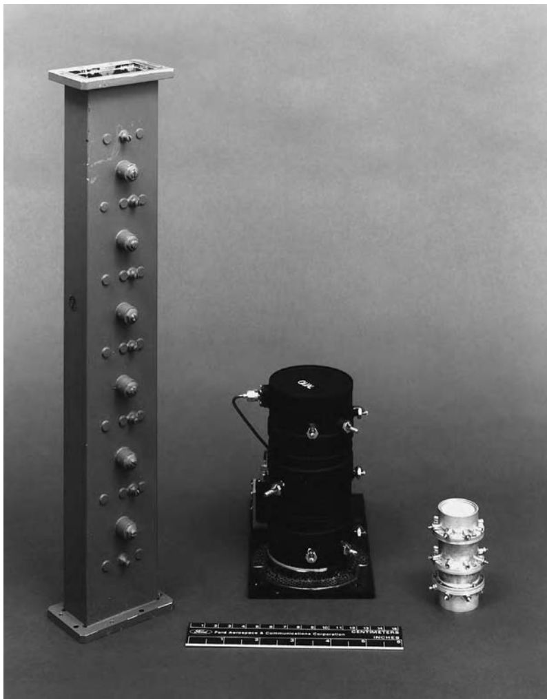
FIGURE 4.11 Size comparisons between traditional cavity filters and dielectric resonator filter (single mode rectangular waveguide filter, dual mode circular cavity filter, and dual mode dielectric resonator filter are shown).
