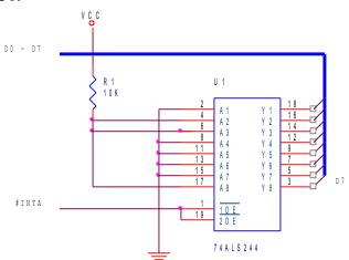
33. The pull-ups force the inputs of the data bus to FFH when the interrupt acknowledge cycle executes.
