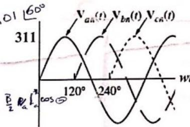
$v_{an}(t) = 311 \sin(314t) \text{ V}$
