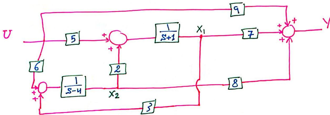
(ii) This Block Diagram Can't be Reduced easily
