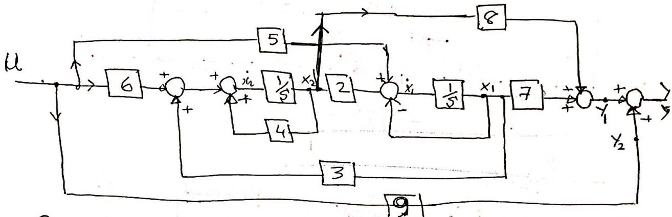
$G_{1(s)} = \frac{Y_1}{U} = \frac{Y_1 + Y_2}{U} = \frac{Y_1}{U} + \frac{9U}{U} = G_{11(s)} + 9$ , so determine  $G_{11(s)}$ . This proves very difficult using reduction techniques. Instead the following has been done to obtain  $G_{11(s)}$ :
