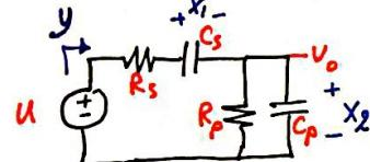
\* T.F could be obtained by two methods:  $G(s) = \frac{Y(s)}{U(s)}$  OR  $G(s) = C \{ sI - A \}^{-1} B + D$
