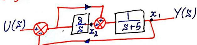
$$X_1(s) = \frac{1}{s+5} (X_2(s) + U(s) - X_1(s)) \Rightarrow \dot{x}_1 = -6x_1 + x_2 + u \quad \dots \textcircled{1}$$
