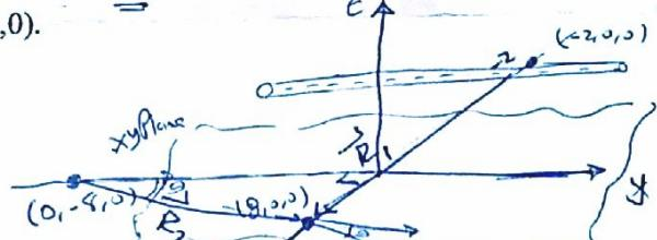
$$\begin{aligned} \vec{R}_2 &= (8, 0, 0) - (-2, 0, 0) \\ \vec{R}_1 &= (8, 0, 0) - (0, 8, 0) \\ \vec{R}_2 &= 8\hat{a}_x \\ \vec{R}_1 &= 8\hat{a}_y \\ \vec{a}_{R_2} &= \frac{\vec{R}_2}{|\vec{R}_2|} \\ \vec{a}_{R_1} &= \vec{R}_1 \sin \theta \hat{a}_x + \vec{R}_1 \cos \theta \hat{a}_y \\ |\vec{R}_2| &= 10 \\ |\vec{R}_1| &= 10 \\ \vec{a}_{R_1} &= \frac{10}{10} \hat{a}_y = \hat{a}_y \end{aligned}$$
