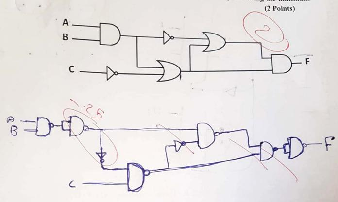
Problem 6: Implement the following function using 3-input OR gates and 3- input AND gates only (2 Points)
