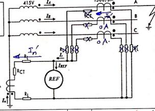
i. Assume a fault of 2000 A fault current develops from the middle parts of the phase winding C of the transformer to the transformer core which is connected to earth, find the CTs secondary phasor currents, residual current, neutral current, and the resultant current in the REF relay  $I_{REF}$ .
