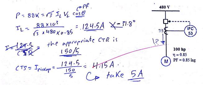
The single-line diagram of a small power system along with its parameters is shown below.
