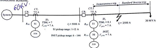
The fault level at the location of  $CB_1$  is 5000A. Strong faults (above 2500A) will be cleared by the instantaneous overcurrent element of  $R_{IN1}$ . Weaker faults towards the end of the feeder ( $\leq 2500$ A) will be cleared by the SI element of  $R_{SI1}$ .
