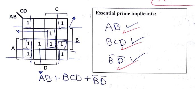
**Problem 5:** Given the following function F: (3.5 points)  $F(A,B,C,D) = \left( (\bar{A} + \bar{C}) \cdot (\bar{B}CD + \bar{A}\bar{B}) \right) + \bar{C}D$
