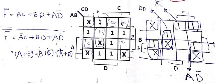
$$F(A,B,C,D) = (A + \overline{C}) \cdot (\overline{B} + \overline{D}) \cdot (\overline{A} + D)$$
