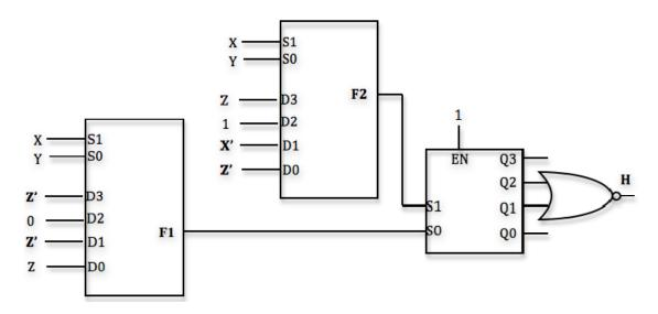
(a) (3 pts) Derive the truth table for the function H (X, Y, Z).
