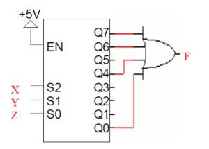
(b) (2 pts) Next, implement F using the decoder shown here and one additional gate
