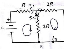
Q6) In the figure, if I = 3.0 A in the circuit segment shown, what is the potential difference  $V_B - V_A$  (in volt)? b) -52 e) +2.0
