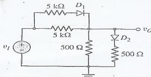
(a) For  $v_i$  small, both diodes are OFF
