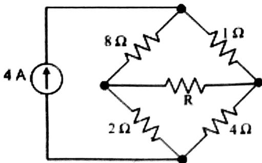
5) If we replace the current source with voltage source with 4V and adjusted R again to absorb maximum power, then R in Ohms is:
