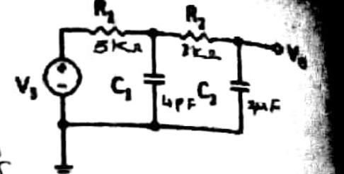
since the resistances  $R_1$  and  $R_2$  are of the same order and  $C_1$  and  $C_2$  are order of magnitude different, then the time constants are well far apart. Hence, the method applies.
