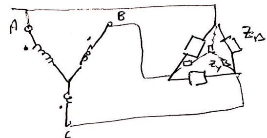
b-If a 3-ph transformer has  $V_{AB}=173.2 / 70^\circ$  kV and  $V_{ab}=10 / 40^\circ$  kV and  $N_{HV}/N_{LV}=10$ , find the connection designation and its vector group. [5]
