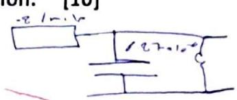
$$60 \% \text{ compensation} = C \frac{B_c}{B_L} \Rightarrow \frac{B_{\text{compensation}}}{1.0305 \cdot 10^{-3} \text{ S}} = .6$$
