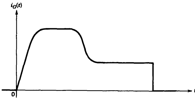
Figure 23-9 A gate current with an initial large value in order to maximize the initial turned-on areas of the thyristor. The current is then reduced to smaller values for a sufficient period of time to guarantee device turn-on.
