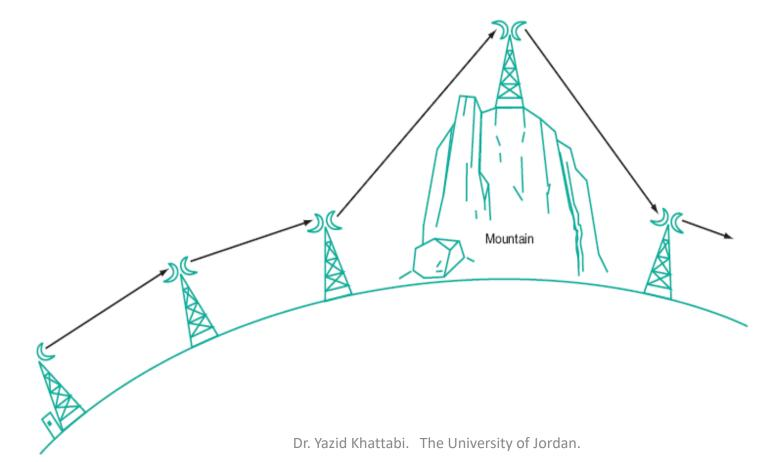
• To increase the range: use a <u>repeater stations</u>. The repeater picks up a signal from a remote transmitter, amplifies it, and retransmits it (on another frequency) to a remote receiver.
