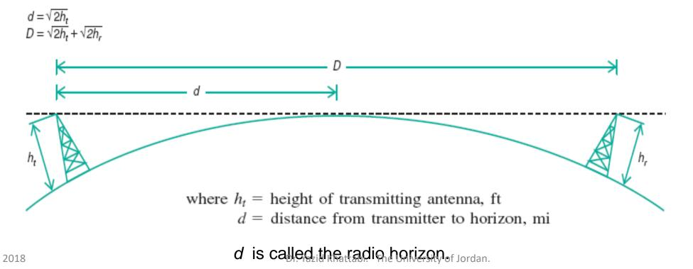
• Transmitting antenna is 350 ft high. Receiving antenna is 25 ft high, the longest practical transmission distance is?
