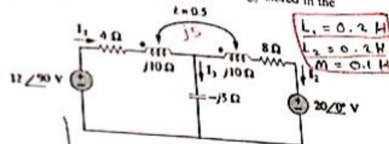
$$\omega(0.1) = \frac{1}{2} L_1 i_1(0.1) + \frac{1}{2} L_2 i_2(0.1) + M i_1(0.1) i_2(0.1)$$
