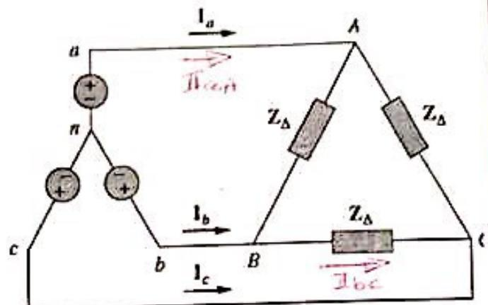
$$\begin{aligned} Z_D &= \frac{V_{AB}}{I_{AB}} = \frac{692.82 \angle +30^\circ}{72.2 \angle -1.79^\circ} \\ &= 9.6 \angle 31.79^\circ \\ &= 8.16 \angle 31.79^\circ \end{aligned}$$
