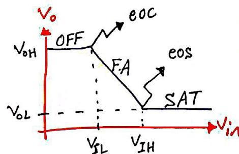
$$\begin{aligned} V_{oH} &= V_{cc} \\ V_{oL} &= V_{CE(sat)} \\ V_{IL} &= V_{BE(on)} \end{aligned}$$
