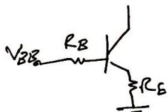
$$I_C = \beta \frac{V_{BB} - V_{BE}}{R_B} \quad \text{and} \quad I_C = \beta \frac{V_{BB} - V_{BE}}{R_C + (1+\beta)R_E} \approx \frac{V_{BB} - V_{BE}}{R_E} \quad (\text{stable}).$$
