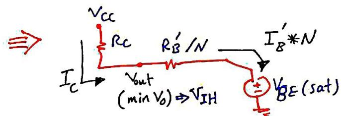
By KVL:  $\frac{V_{cc} - V_{out}}{R_c} = I_C$ ,  $I_B' = \frac{V_{cc} - V_{BE(sat)}}{R'_B \cdot \beta}$ ,  $I_C = N I_B'$
