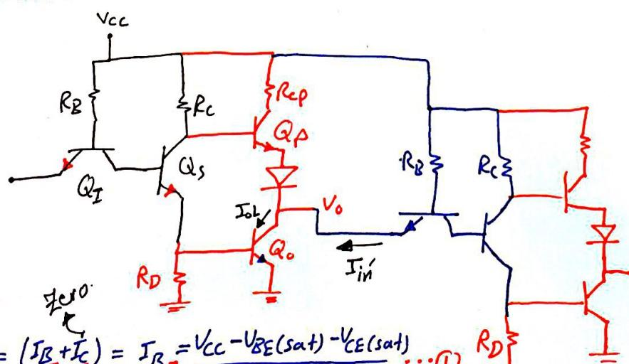
$$I_{D'} = (I_B + I_C) = I_B \cdot \frac{V_{CC} - V_{BE(sat)} - V_{CE}}{R_B}$$
