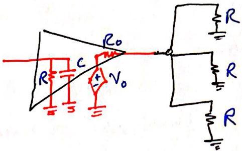
problem: that the  $\underline{z}$ -resistances are in parallel which decrease  $R_{eq}$  which increase the drawn current which lead to increase the voltage drop on  $R_o$  if  $V_o = 5V$ ,  $V_{R_o}$  would take  $3V$  which logically will become zero voltage at the output. since we will have  $2V \equiv \text{Logic 0}$ .
