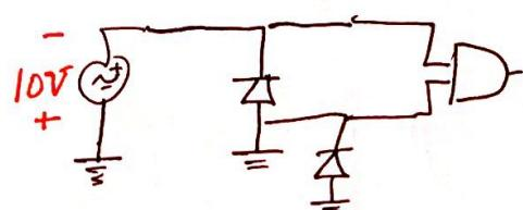
if we input a  $-10\text{V}$  the diode will be reversed-mode & it will output a  $0.7\text{V}$ .
