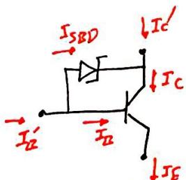
$$I_C = I_B' + I_{SBD} = \beta I_B \\ = \beta (I_B' - I_{SBD})$$
