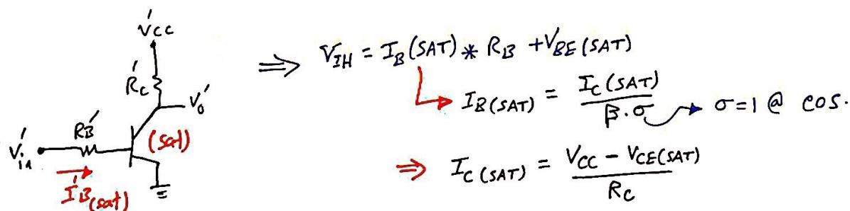
$N$  is max when  $V_{out} = V_{IH}$
