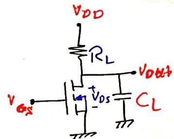
• Case I:  $I_{R_L} = I_{C_L}$        $\frac{V_{DD} - V_o}{R_L} = C_L \frac{dV_o}{dt}$
