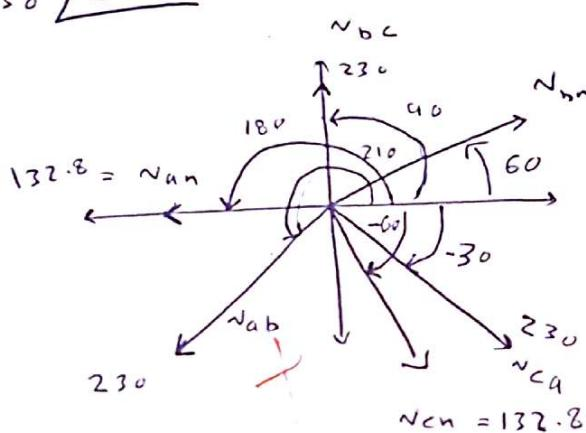
$$V_{an} = 132.8 \angle 180^\circ$$
