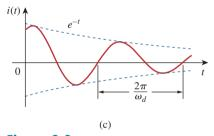
**Figure 8.9**(a) Overdamped response, (b) critically damped response, (c) underdamped response.
