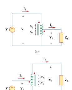
**Figure 13.42**(a) Step-down autotransformer, (b) step-up autotransformer.
