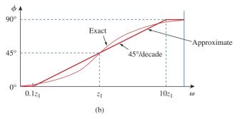
**Figure 14.11** Bode plots of zero  $(1 + j\omega/z_1)$ : (a) magnitude plot, (b) phase plot.
