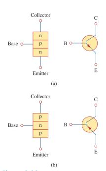
**Figure 3.38** Two types of BJTs and their circuit symbols: (a) *npn*, (b) *pnp*.
