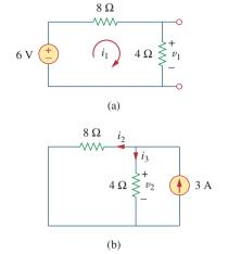
**Figure 4.7** For Example 4.3: (a) calculating  $v_1$ , (b) calculating  $v_2$ .
