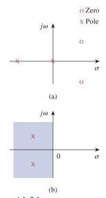
**Figure 16.26** The complex *s* plane: (a) poles and zeros plotted, (b) left-half plane.
