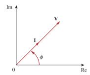
Figure 9.10 Phasor diagram for the resistor.
