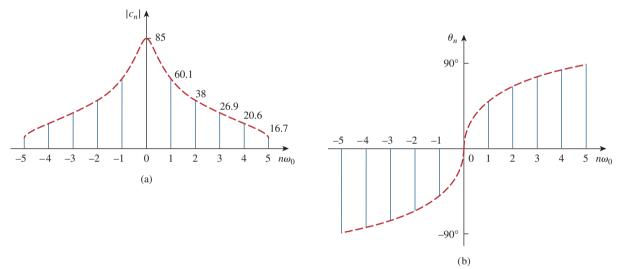
**Figure 17.30**The complex frequency spectrum of the function in Example 17.10: (a) amplitude spectrum, (b) phase spectrum.
