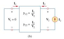
**Figure 19.12** Determination of the *y* parameters: (a) finding  $y_{11}$  and  $y_{21}$ , (b) finding  $y_{12}$  and  $y_{22}$ .
