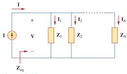
**Figure 9.20** *N* impedances in parallel.
