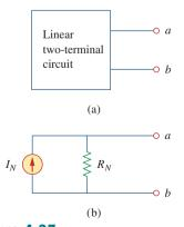
**Figure 4.37**(a) Original circuit, (b) Norton equivalent circuit.
