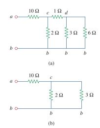
**Figure 2.38** Equivalent circuits for Example 2.10.
