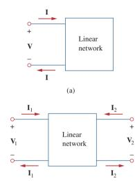
**Figure 19.1**(a) One-port network, (b) two-port network.
