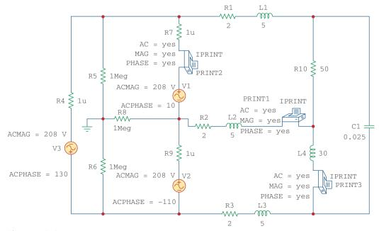
**Figure 12.31** Schematic for the circuit in Fig. 12.30.
