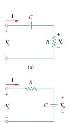
**Figure 9.31**Series *RC* shift circuits: (a) leading output, (b) lagging output.
