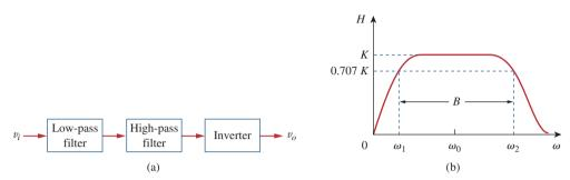
**Figure 14.44** Active bandpass filter: (a) block diagram, (b) frequency response.
