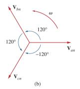
**Figure 12.7** Phase sequences: (a) *abc* or positive sequence, (b) *acb* or negative sequence.
