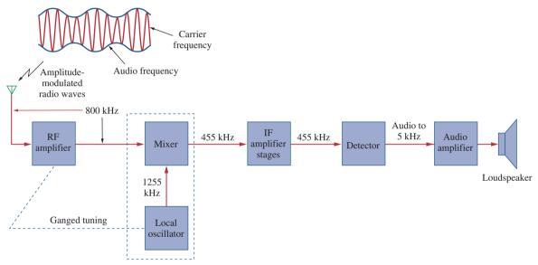
**Figure 14.62** A simplified block diagram of a superheterodyne AM radio receiver.
