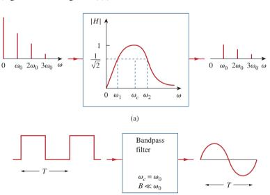
**Figure 17.44** (a) Input and output spectra of a bandpass filter, (b) the bandpass filter passes only the fundamental component when  $B \ll \omega_0$ .
