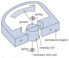
**Figure 2.58** A d'Arsonval meter movement.
