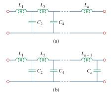
**Figure 19.61** *LC* ladder networks for lowpass filters of: (a) odd order, (b) even order.
