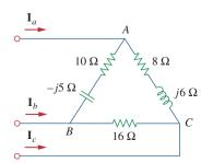
**Figure 12.24** Unbalanced  $\Delta$ -load; for Practice Prob. 12.9.
