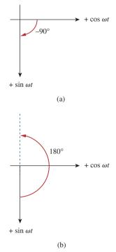
**Figure 9.3** A graphical means of relating cosine and sine: (a)  $\cos(\omega t - 90^{\circ}) = \sin \omega t$ , (b)  $\sin(\omega t + 180^{\circ}) = -\sin \omega t$ .
