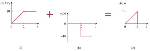
**Figure 7.37** Complete decomposition of v(t) in Fig. 7.35.
