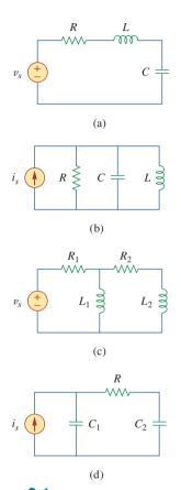
**Figure 8.1** Typical examples of second-order circuits: (a) series *RLC* circuit, (b) parallel *RLC* circuit, (c) *RL* circuit, (d) *RC* circuit.
