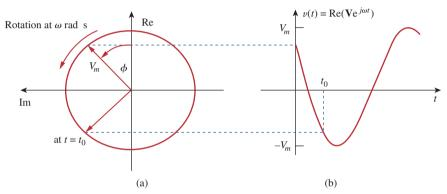
**Figure 9.7** Representation of  $Ve^{j\omega t}$ : (a) sinor rotating counterclockwise, (b) its projection on the real axis, as a function of time.
