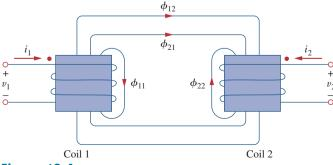
**Figure 13.4** Illustration of the dot convention.
