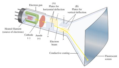
**Figure 1.17** Cathode-ray tube.
