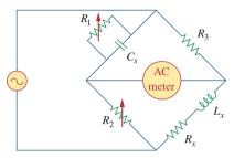
**Figure 9.84**Maxwell bridge; For Prob. 9.84.
