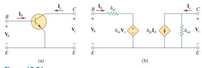
**Figure 19.56**Common emitter amplifier: (a) circuit schematic, (b) hybrid model.
