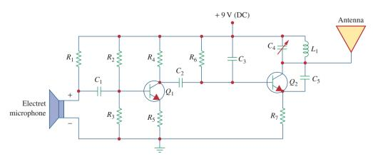
**Figure 1.2** Electric circuit of a radio transmitter.
