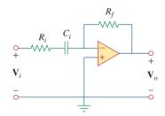
**Figure 14.43** Active first-order highpass filter.
