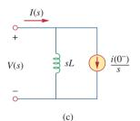
**Figure 16.1** Representation of an inductor: (a) timedomain, (b,c) *s*-domain equivalents.
