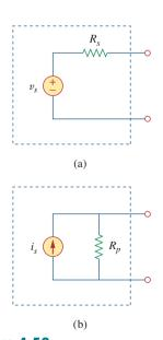
**Figure 4.58**(a) Practical voltage source, (b) practical current source.
