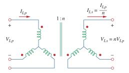
**Figure 13.46** Y-Y three-phase transformer connection.
