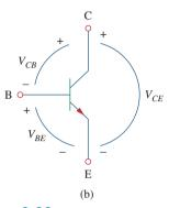
**Figure 3.39** The terminal variables of an *npn* transistor: (a) currents, (b) voltages.
