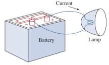
**Figure 1.1** A simple electric circuit.
