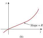
**Figure 2.7** The *i-v* characteristic of: (a) a linear resistor, (b) a nonlinear resistor.
