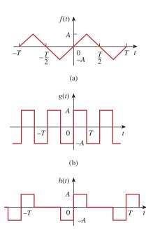
**Figure 17.11** Typical examples of odd periodic functions.
