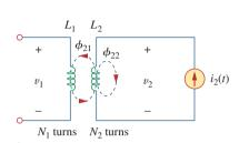
Figure 13.3 Mutual inductance  $M_{12}$  of coil 1 with respect to coil 2.
