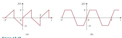
**Figure 17.12**Typical examples of half-wave odd symmetric functions.
