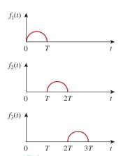
**Figure 15.4** Decomposition of the periodic function in Fig. 15.3.
