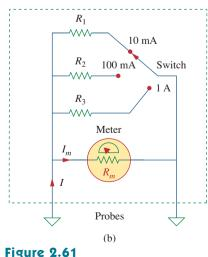
Ammeters: (a) single-range type, (b) multiple-range type.
