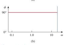
**Figure 14.10** Bode plot for a zero  $(j\omega)$  at the origin: (a) magnitude plot, (b) phase plot.
