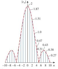
**Figure 17.28**The amplitude of a periodic pulse train.
