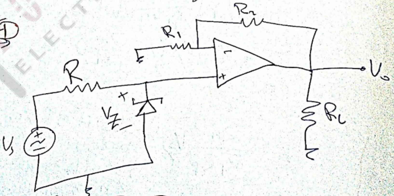
$$V_o = \left(1 + \frac{R_2}{R_1}\right) V_Z = V_L \quad \#$$
