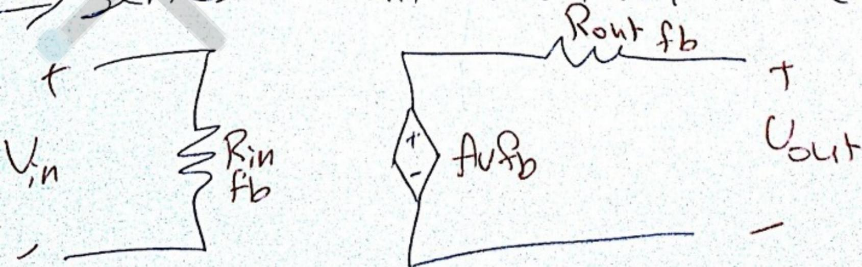
where  $R_{in_{fb}}$ ,  $R_{out_{fb}}$ ,  $A_{V_{fb}}$  as the up equation.
