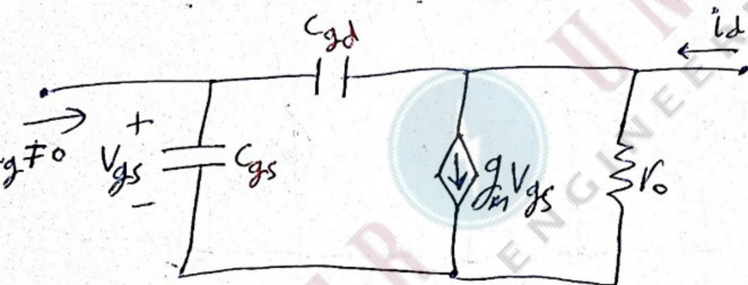
⇒ short circuit current gain  $(A_i) = \frac{i_d}{i_g}$
