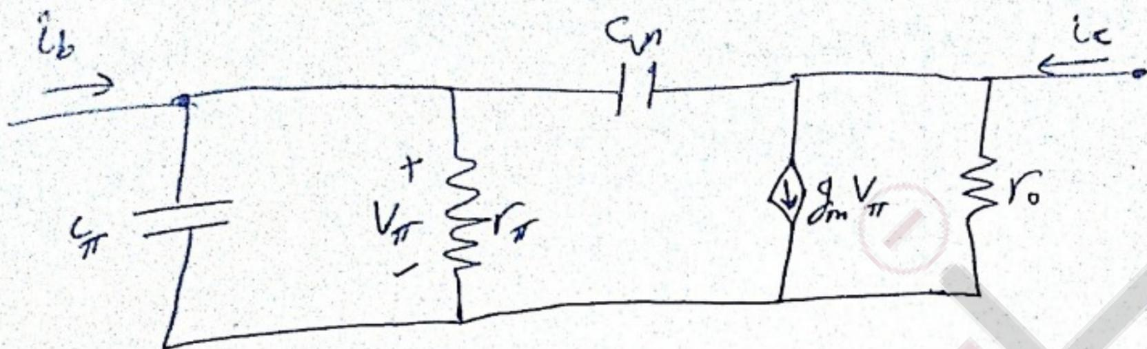
$C_{\pi}$  :- Forward-biased Junction capacitor
