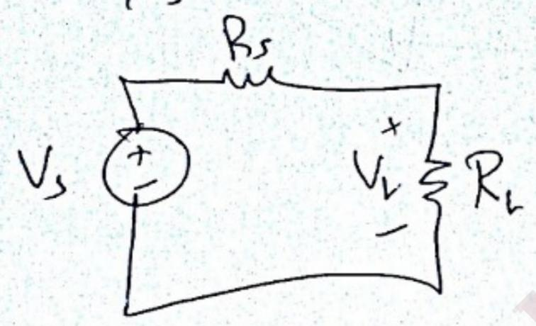
$$\Rightarrow V_L = V_s \frac{R_L}{R_L + R_S}$$
