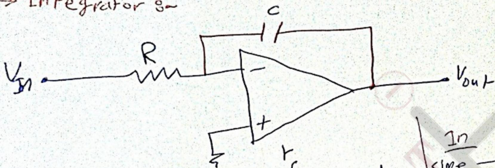
$$V_{out}(t) = V_c - \frac{1}{RC} \int_0^t V_{in}(t) \cdot dt$$
