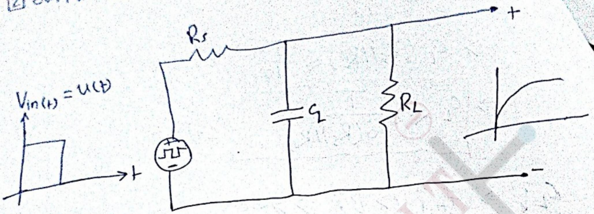
$$\frac{V_o(s)}{V_{in}(s)} = K * \frac{1}{1+s\tau} \quad \text{where } \tau = C_L (R_S \parallel R_L)$$
