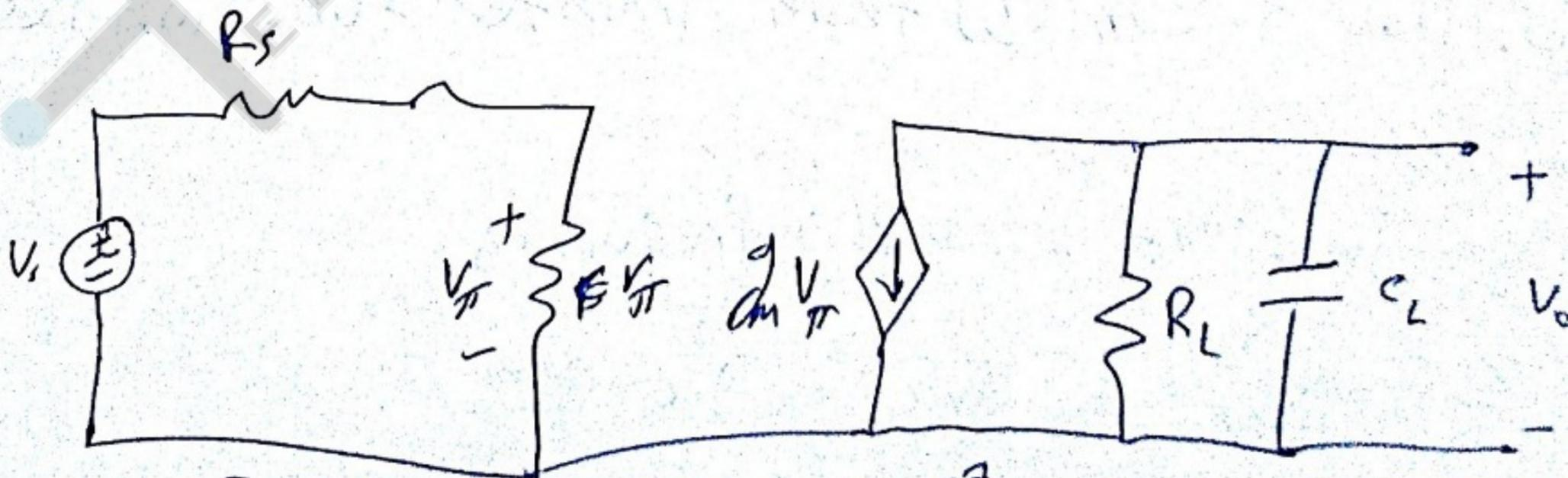
$$T = R_{th} C_c = C_c \times R_L = 2 \times 10^{-7} \text{ sec}$$
